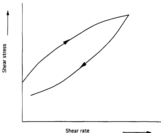
Figure 10.33 Representation of shear stress as a function of shear rate for yoghurt displaying rheological hysteresis.
